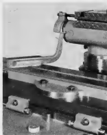
Figure 27A Centering Gage on Table Indicating Zero-Mark on Wheelhead
